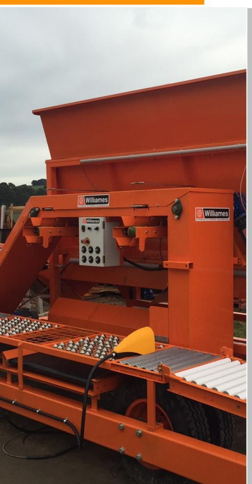
Galvanised Steel Roller Conveyors flank Two Stainless Steel Transfer Ball Stations (each placed beneath the soil feeder chute).
