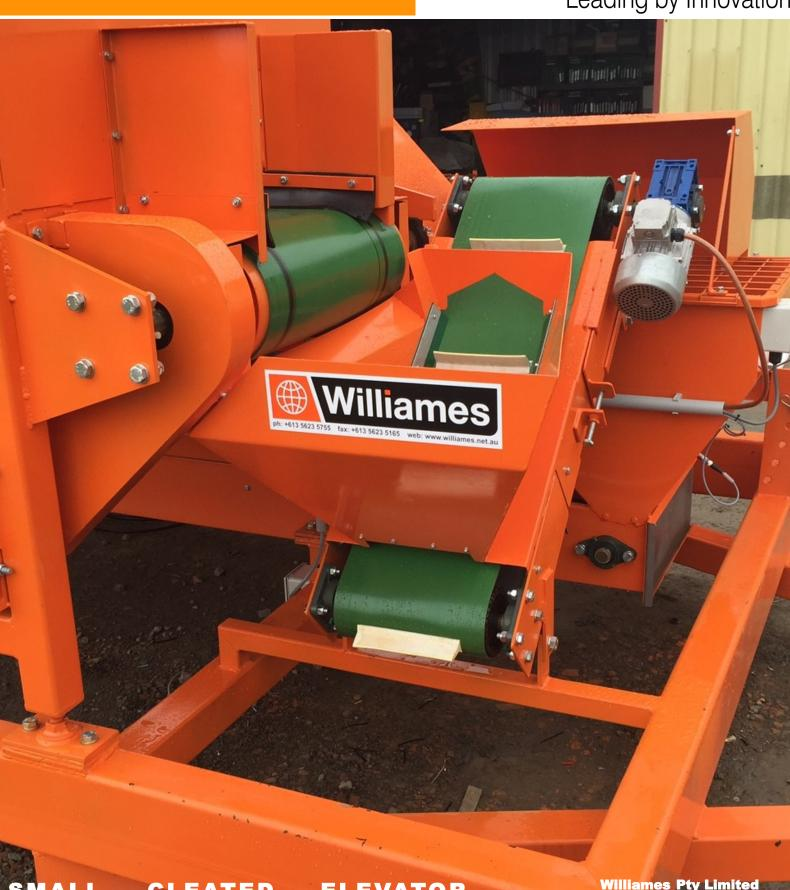
SMALL CLEATED ELEVATOR CONVEYOR
