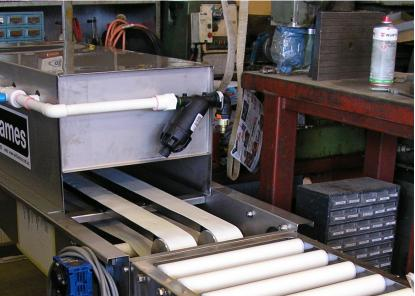
BELT CONVEYOR OF TWO WHITE POLYURETHANE STRIPS DRAINS WATER AWAY QUICKLY ... white plastic roller conveyor doesn't carry the water into work area DC Watering Tunnel
