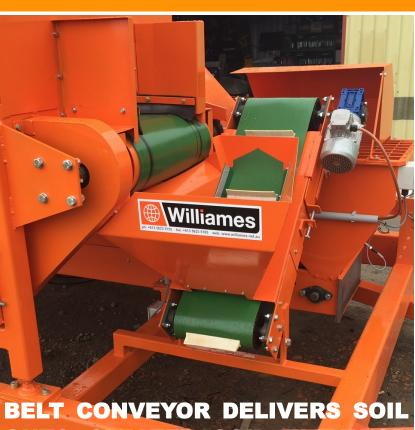
ONTO CLEATED SOIL ELEVATOR POT FILLER SHUTES TO RAPIDLY FILL VERY LARGE POTS ... part of Transportable Pot Filler
