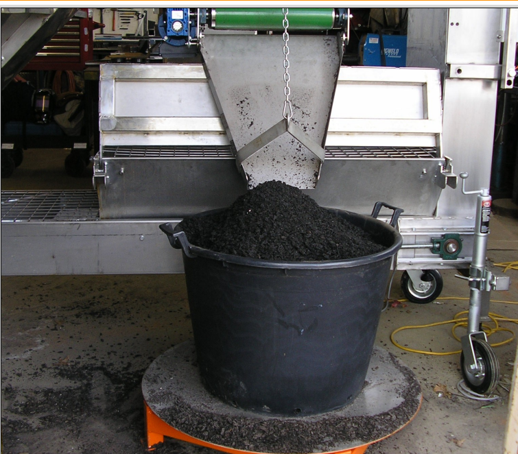
[1] Williams Multipurpose S/S Pot & Bag Filler can fill 800MM pots & bags rapidly and safely either on the stainless steel wire-mesh bench ( above right ) or effortlessly on a turntable on the floor that can be easily turned while the fill is delivered in a controlled-flow stream via an extended S/S Soil Chute ( above ).
