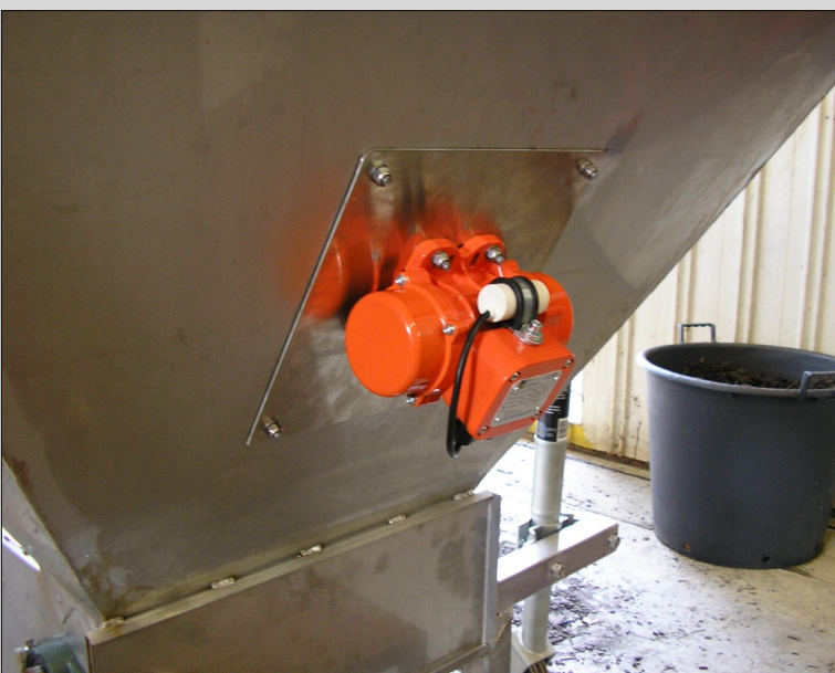
[2] Williams Bin Vibrator ( above ) on the outside of the soil bin is used if the soil mix becomes compacted in the bin. This is more common with a 'fluffy' loose mix containing shredded bark than with a finely textured mix.
