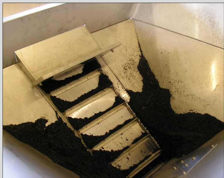
[4] Williams Soil Elevator & Inbuilt Soil Return ( above ) carries the soil up to the horizontal soil exit and falls onto the Soil Feed Conveyor which delivers the fill to the pots or bags below via the Soil Feed Shute ( above left ). Excess soil falling off the bench is carried back to the bin.
