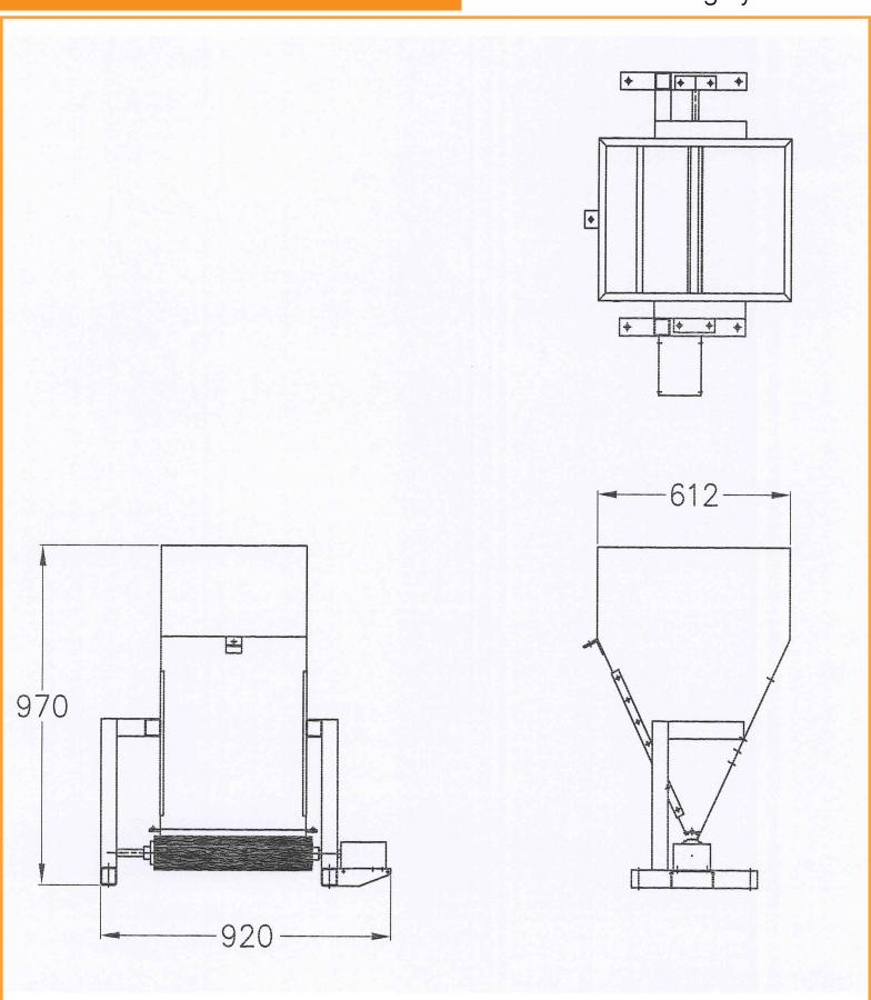
V2 VERMICULITE COVER: SIDE ELEVATION END ELEVATION AND PLAN
