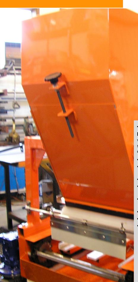
The Williames V2 Covering Machine adds a covering layer (i.e., vermiculite) after the tray has been filled and seeded. The V2 dispenses an even layer of cover.
