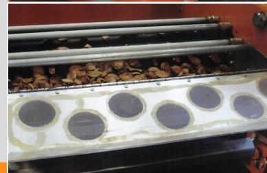
**V2 VERMICULITE COVERER** adds a covering layer to the tray (i.e., layer of vermiculite) after the tray has
