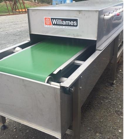
**DC WATERING TUNNEL** waters trays after they been filled, seeded and covered. Water is sprayed across the tray as it passes underneath.
